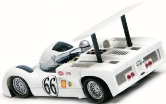
In 1966 Chaparral introduced model 2E for the Can-Am series. With its high mounted wing, clever aerodynamics and rear mounted radiators, it was the car that changed racing, forever. Its best result was at Laguna Seca, where the 2E of Phil Hill won the race and Jim Hall finished second.
